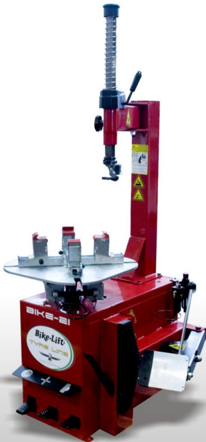
*Semi-automatic tyre changer, designed to mount and demount motorcycle, mopeds, ATV, Quads, Go karts and turf vehicles.*
